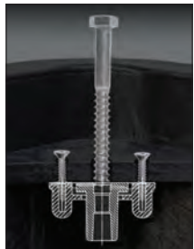
Non-Seizing Bolt System Allows Field Replacement
